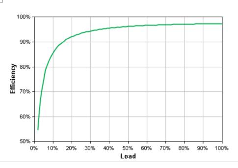
Curve fit to measured efficiency data. All measurements taken in normal operating mode, at typical environmental conditions, with nominal electrical input and balanced resistive load (PF = 1.0) output.
